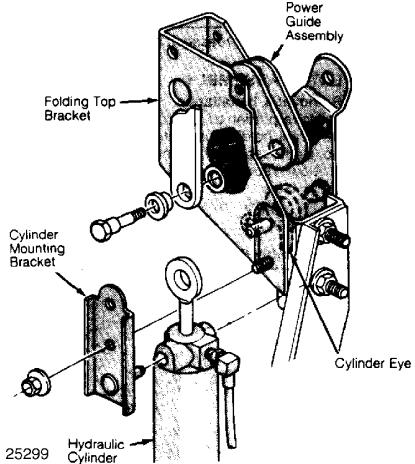
Fig. 2: Hydraulic Cylinder & Mounting Bracket Courtesy of Chrysler Motors.
