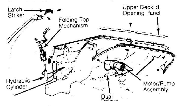
Fig. 1: LeBaron Power Top Component Location Courtesy of Chrysler Motors.
